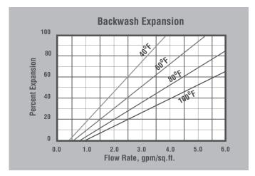
**BACKWASH** — The backwash step is used to separate the components prior to regeneration and to remove particles. The separation is optimized at a bed expansion of 50 to 75 percent.
